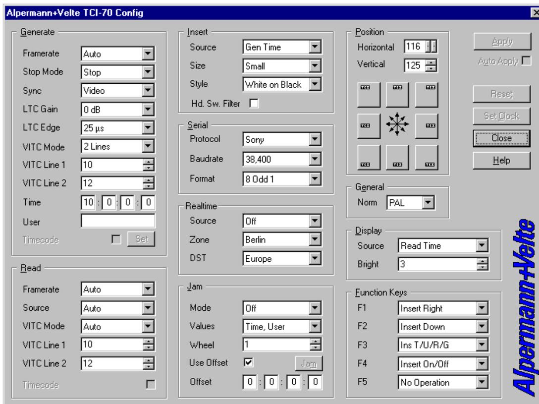
All configuration settings are displayed here. If you change one of the preset information it will not have any effect on the TCI-70. Only if "Apply" is pressed the change will be submitted to the TCI-70. That way you can experiment with the settings first without interfering with the current operation. If all changes shall be submitted to the TCI-70 immediately mark "Auto Apply".
