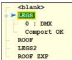
Figure 6- Controller 'LEGS' connected to DMX controller 0
