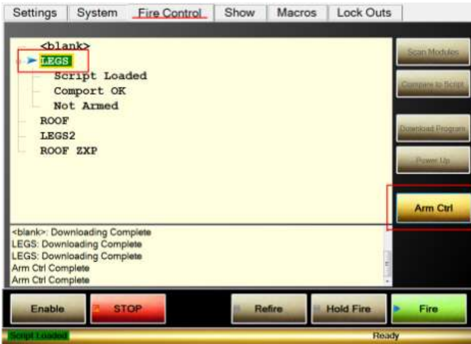
Figure 7- Fire Control screen ready to Arm controller LEGS
