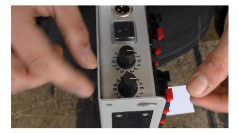
8. Use a Controller to double-check that the Shaft is in the correct position.
