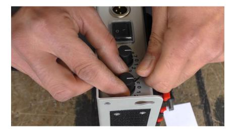
2. Take the assembly tool and screw of the knob. Important: Don't adjust the shaft to a different adress! Ensure the shaft is in Position 00! To check if the shaft is on 00, the flat side have to show down, or check it with a Controller
