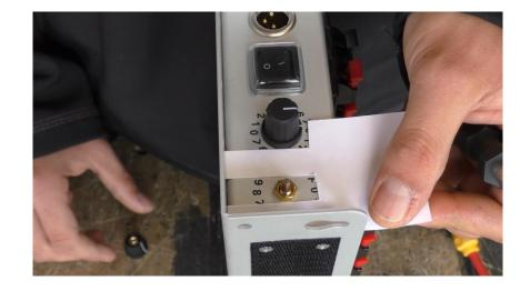
4. Put the knob exactly with the white line to the 0 Position
