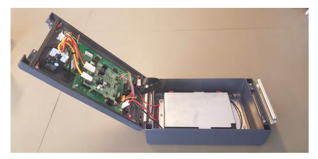
Detach the main fuse. You can easily identify the main fuse by its yellow color.
