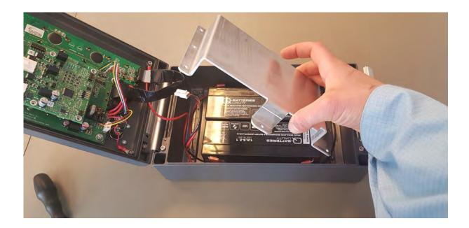
Now, take out the battery pack with its cables still attached.
