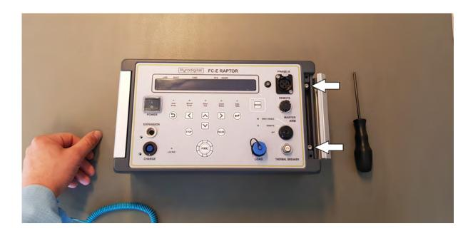
Tighten the two screws on the right and close the cover.
