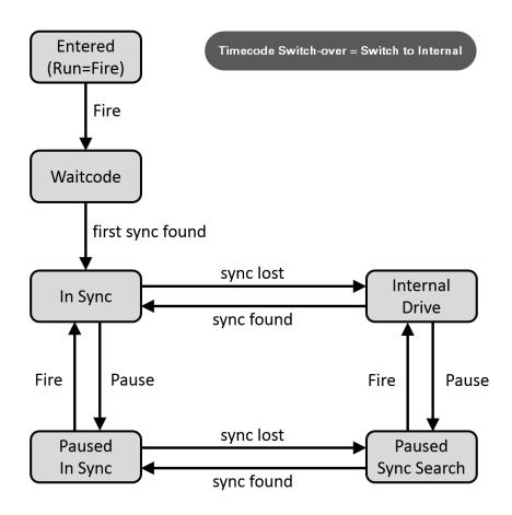
First the Operator has to depress FIRE to proceed to the 'Waitcode' state. Then, after the first valid timecode frame is received, the clock is 'In Sync' to the timecode. If the timecode gets lost or invalid ('sync lost'), the clock switches over to the internal clock source 'Internal Drive'. When the timecode resumes (and is valid), the clock is resynchronized and again 'In Sync'.
