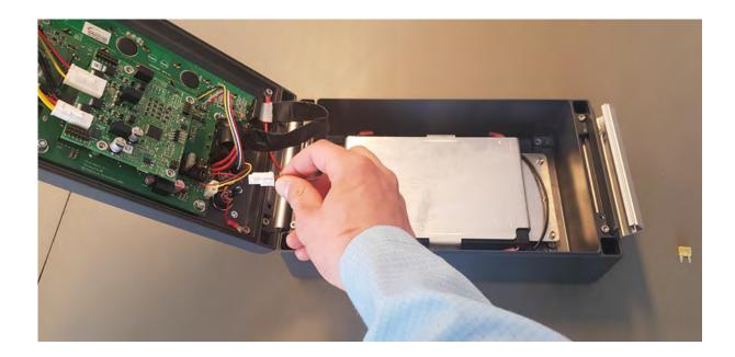
Unscrew the battery holder with a TX20 screwdriver.
