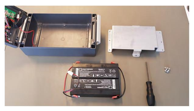
Unplug the Battery Interconnection Cable. Afterwards detach the Main Battery Cable.
