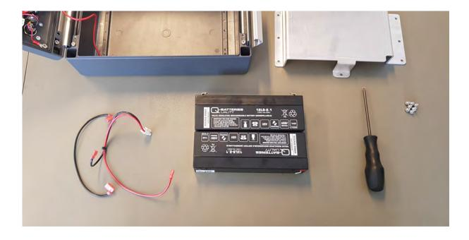
Replace the old batteries for endorsed ones by Innovative Pyrotechnik GmbH (Always endorsed: Q-Batteries 12LS-2.1). Use self-adhesive EPDM Sponge Rubber Foam to fill the small gap inbetween the batteries and holder to secure pressure to the holder. To connect the replaced batteries
