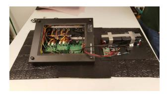
Lay down the housing next to the bottom plate as show in the image above.
