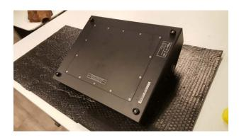
Place the Field Controller bottom up on a soft underground. Unscrew all 14 bottom screws.
