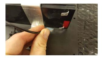
Unplug the Battery Interconnection Cable from the positive pole of the right hand side battery.
