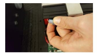
Unplug the Battery Plus Cable from the positive pole of the left hand side battery.
