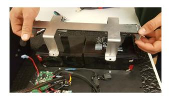
Lift off the holder. The batteries are free now.
