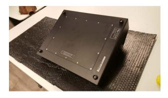
Use the prepared screws wrapped with PTFE Thread Seal Tape to close the Field Controller.
