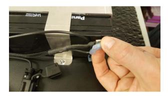
Unplug the Battery Minus Cable from the negative pole of the right hand side battery. Be very careful unplugging this connector as it includes also the temperature sensor of the battery. DO UNPLUG THE WHOLE PART INCLUDING THE SENSOR FROM THE BATTERY.
