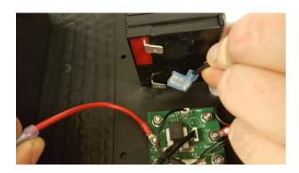
Unplug the Battery Interconnection Cable from the negative pole of the left hand side battery. Be careful to not harm the PCB board next to it and the cables connected to it.
