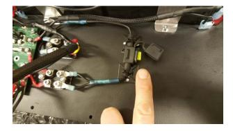
Plug in the Main Fuse before closing the device.
