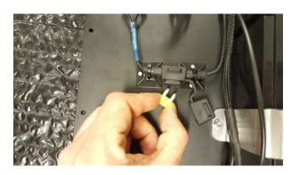
IMPORTANT: Before proceeding any further disconnect the main fuse!!! You successfully opened the Field Controller.
