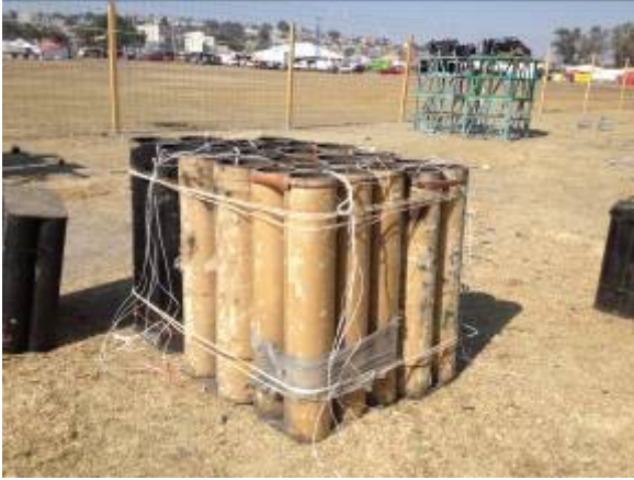
Figure 6 - A bundle of 8” guns unsecured
